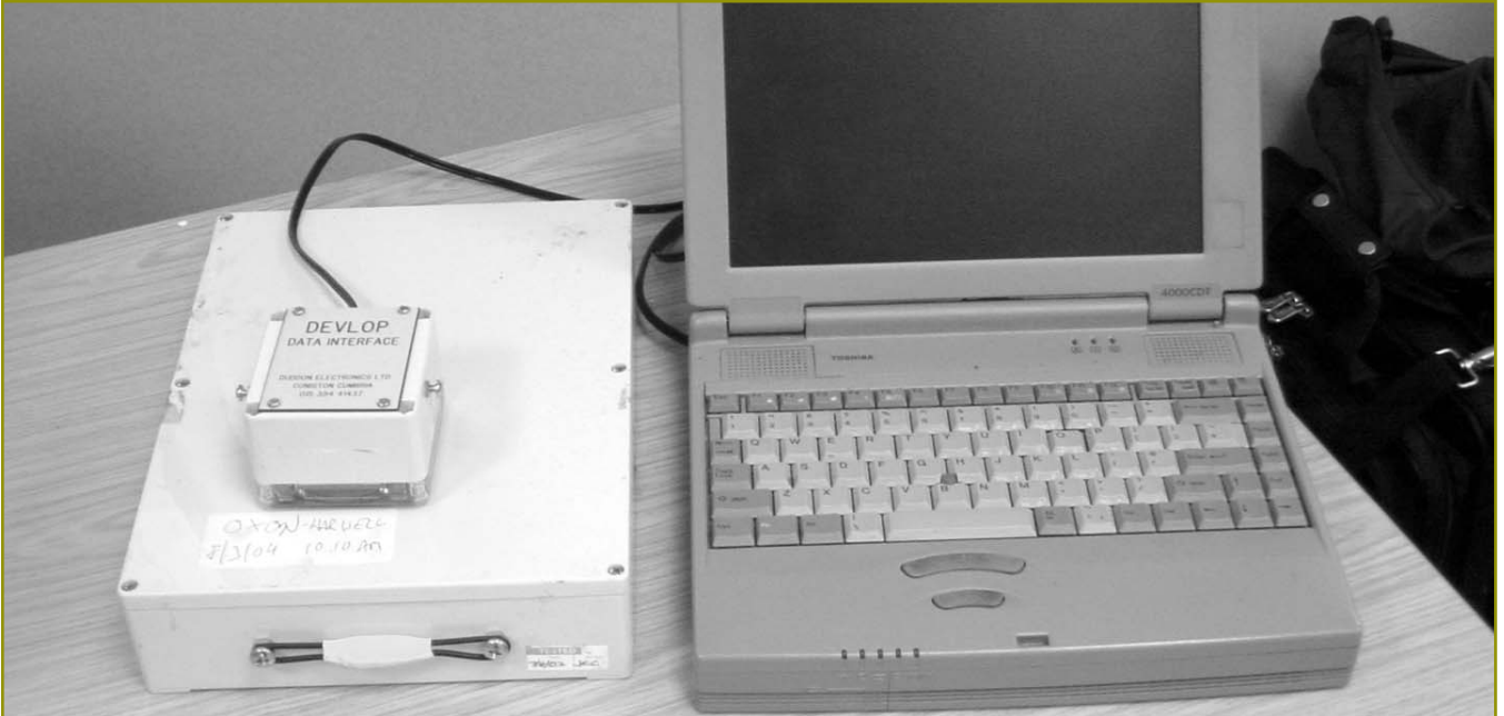
Figure 2.1a: Duddon Electronics vehicle logger at left connected to laptop personal computer at right using DEVLOP interface
